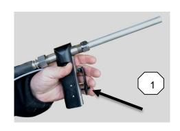
Nozzles can be changed by unfasten the nut that holds the nozzle. Replace the nozzle and fasten the nut again. Hand tight only. No need for tools
