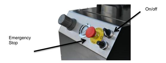
Turn the on/off switch to the right to turn on the machine and left to switch off.
